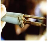
Figure 2 On-tool extraction – soldering iron
